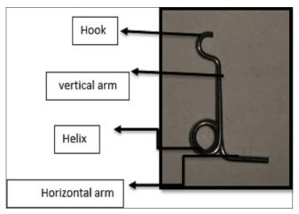
Figure 1: The spring consists of: 1- a horizontal arm, 2- a helix, 3- a vertical arm, 4- a hook
