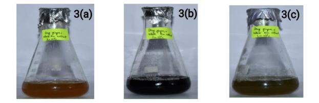
**Figure:** 3(a) Dilution of Zirconium nanoparticles, 3(b) Dilution of Gold nanoparticles, 3(c) Dilution of Copper nanoparticles with dry ginger and white tea extract.
