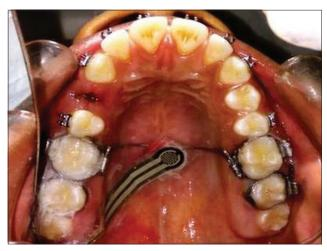
Figure 3: Placement of pressure sensor on acrylic button in the patient's mouth
