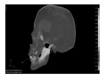
Figure 3: Tensile stress distribution
